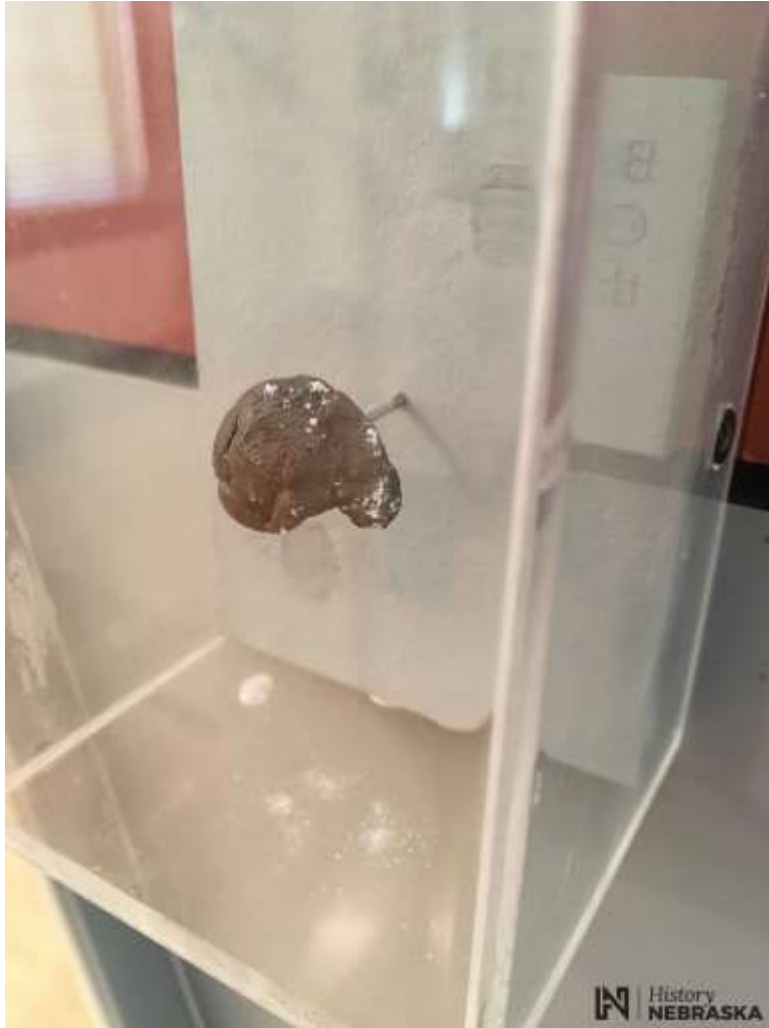
Photo of Bullet in Case with White Lead Corrosion Product Residue
