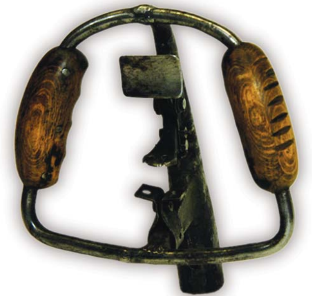
The control stick from Ralston's Sopwith Camel. He carved a notch for each enemy plane he shot down. NSHS 10091-15
