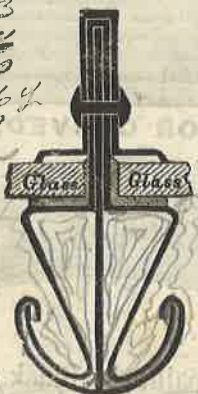
SECTION SHOWING ONE STYLE OF SASH BAR.
