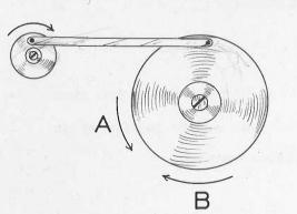
When the little wheel turns around, the big wheel will: A—turn in direction A,
