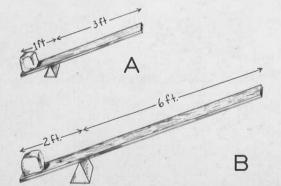
With which arrangement can a man lift the heavier weight?
