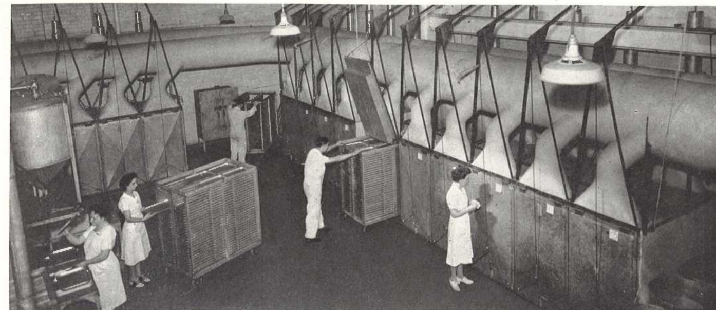
Albumen solubles being dried in air conditioned ovens at a temperature of 110 to 120 degrees Fahrenheit.
