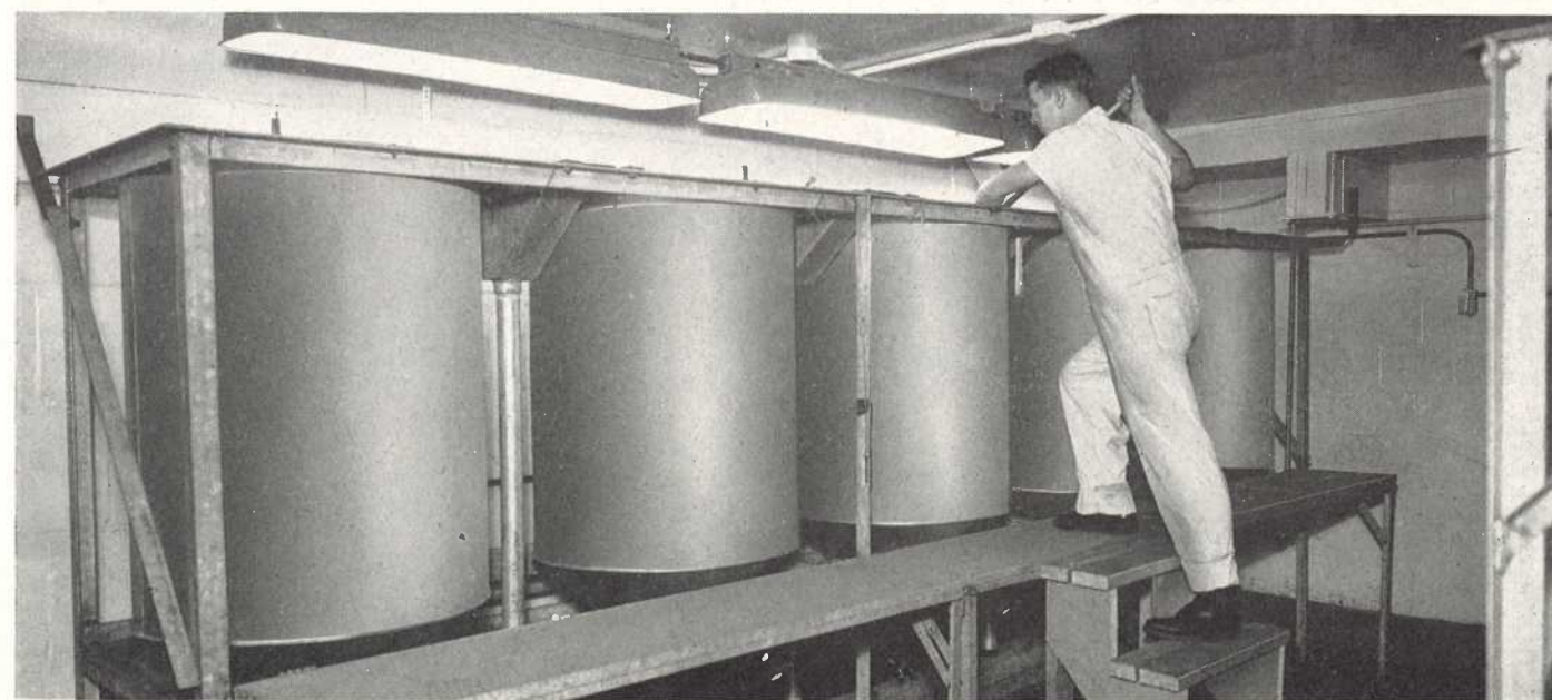
Albumen undergoing treatment by which the unsoluble protein is converted to the soluble form.
