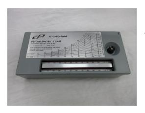
A psychrometer is the most reliable instrument for determining relative humidity, if used properly. It is used to measure daily readings, to make spot readings, and most importantly for calibrating other devices. The psychrometer consists of two thermometers; one that measures the ambient temperature and another that has a moistened sock over the bulb and measures the "wet bulb" temperature. The wet bulb temperature will be lower than the dry bulb temperature because the moistened bulb is
