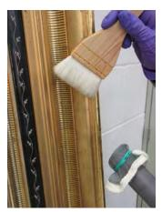
Note the location and power of the exhaust port on the vacuum. It is important to be aware of this port, as air blown out of the vacuum can knock small or light objects off tables or blow them over.
